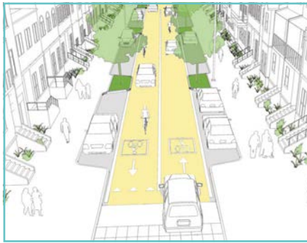
2. Two-Way Street, Narrowed Lanes
