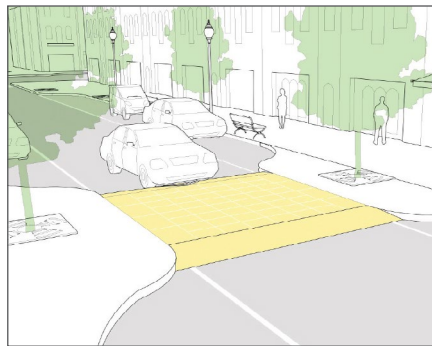
8. Speed Tables/Elevated Crosswalks
