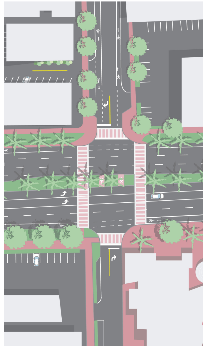
Fig 2.16 Pedestrian crossings should be highly visible. Paint or a simple design throughout the cross walk is a cost-effective way to achieve high visibility.
