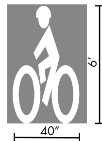
Fig. 2.31 Pavement marking dimensions.
